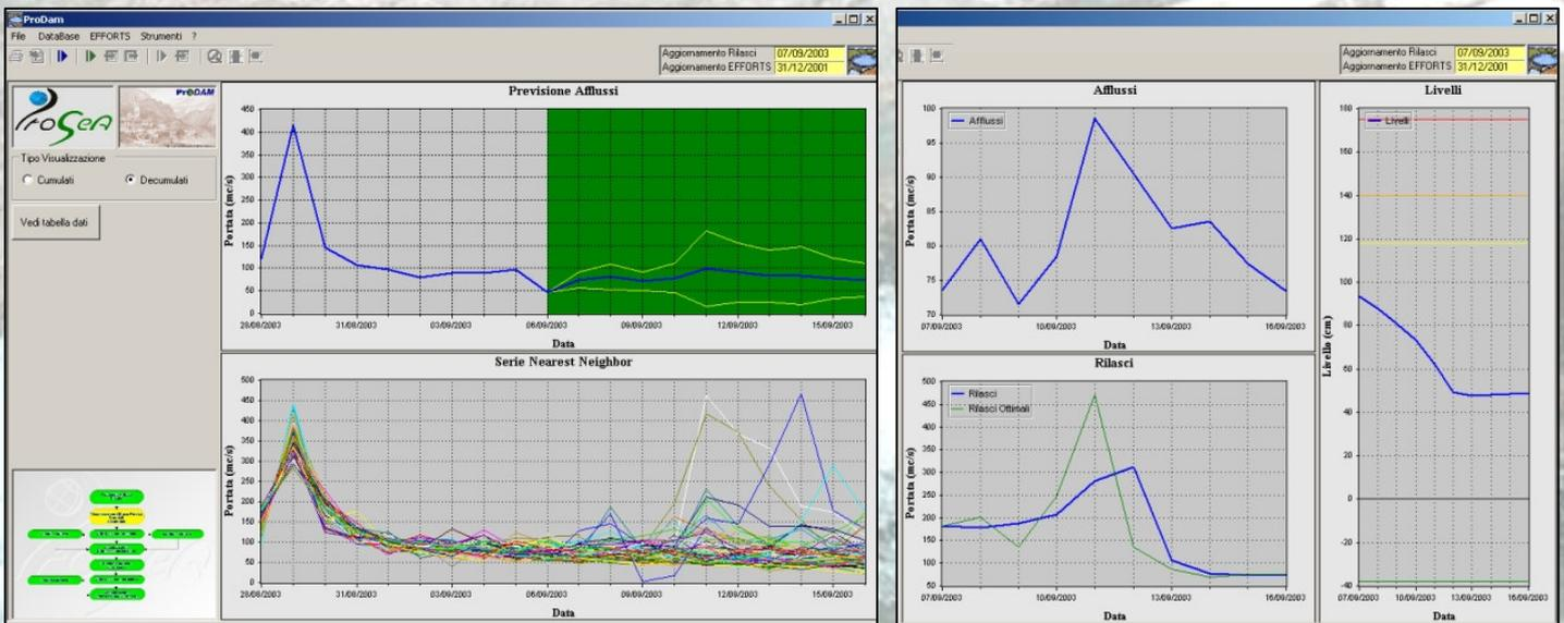
Example of PRODAM visualizations. The panels show forecasted inflow (on the left) and data from the reservoir (on the right): measured inflow, outflow and water level.
